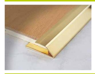
The WOODTEC LP profiles are specifically designed for finishing the perimeter of floating wood floors. The pointed, sloping shape of this profile ideally transitions to existing flooring or floors at lower elevations. The internal gap acts allows for differential movement. Installed with flathead screws.
